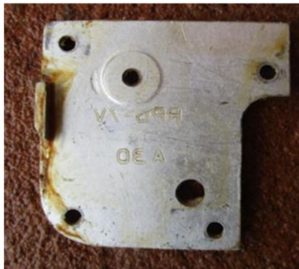
Rear view of the aluminium plate covering the percussion mechanism.
